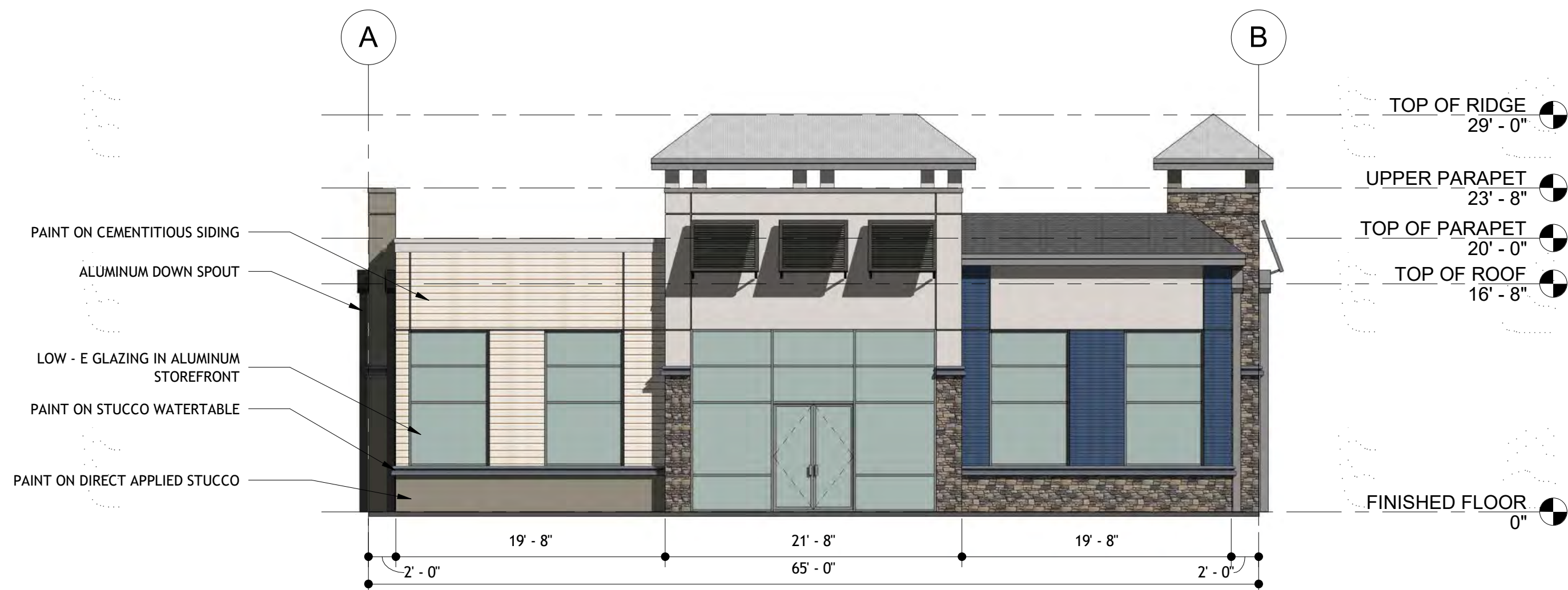
2 SOUTH ELEVATION BUILDING - 1 1/8" = 1'-0"
