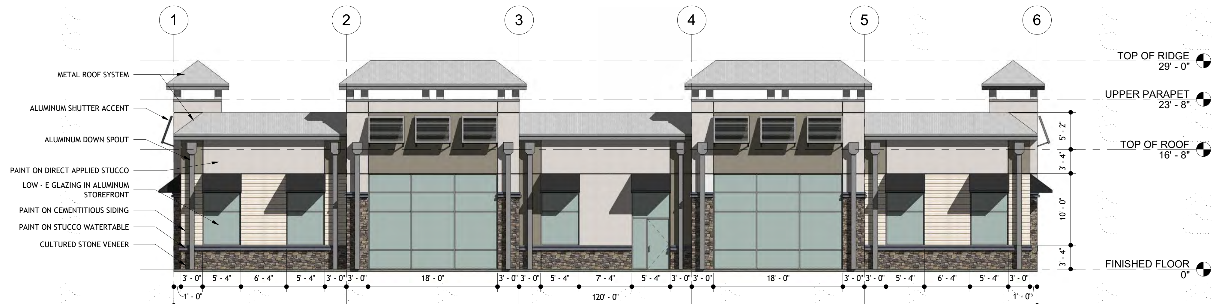
3 EAST ELEVATION BUILDING - 3 1/8" = 1'-0"
